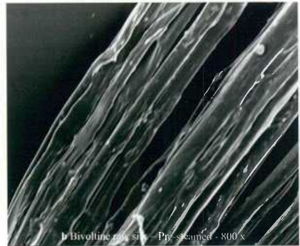
Figure 5: SEM images of bivoltine raw silk, without steaming (a) and after pre-steaming (b)
