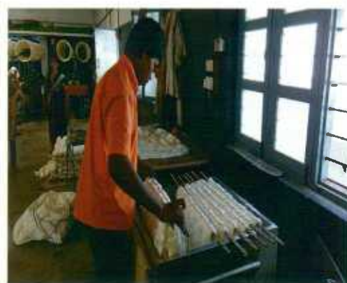
Figure 2: Skeins are placed in the pre-steaming cabinet
