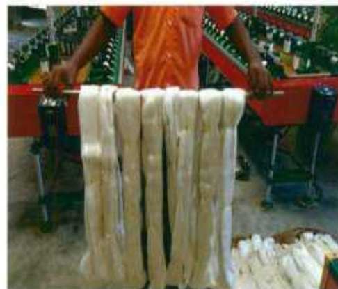
Figure 1: Skeins are arranged for pre-steaming
