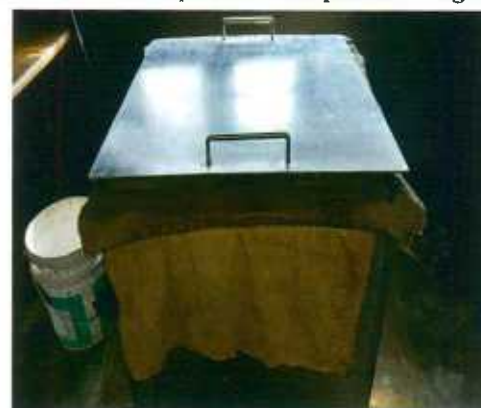
Figure 3: Pre-steaming of raw silk under progress
